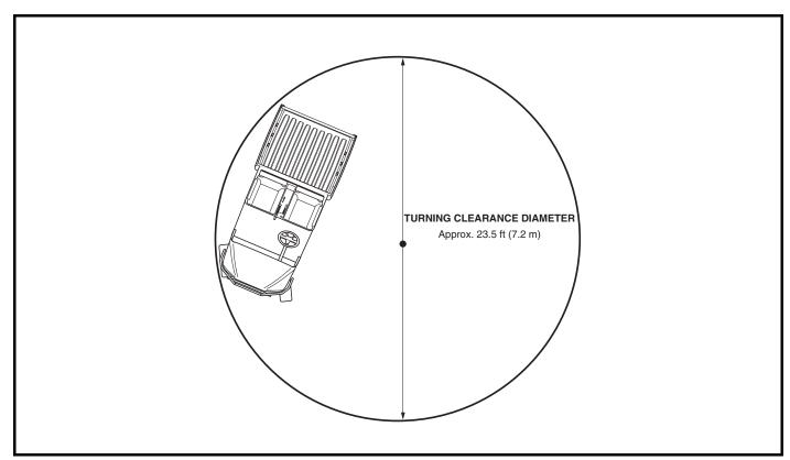
Fig. 3 Vehicle Turning Clearance Diameter
